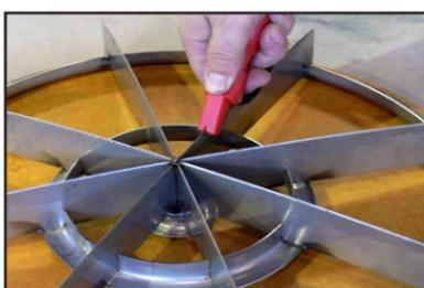
Designed to work best sharp, blades need to be resharpened after cutting 2000 pizzas. Make 2-3 firm strokes across each blade using the hand tool. Sharpening leaves metal burrs; keep away from food area.
