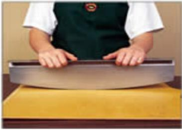
A rocker knife is a curved blade designed to cut by rocking back and forth.
